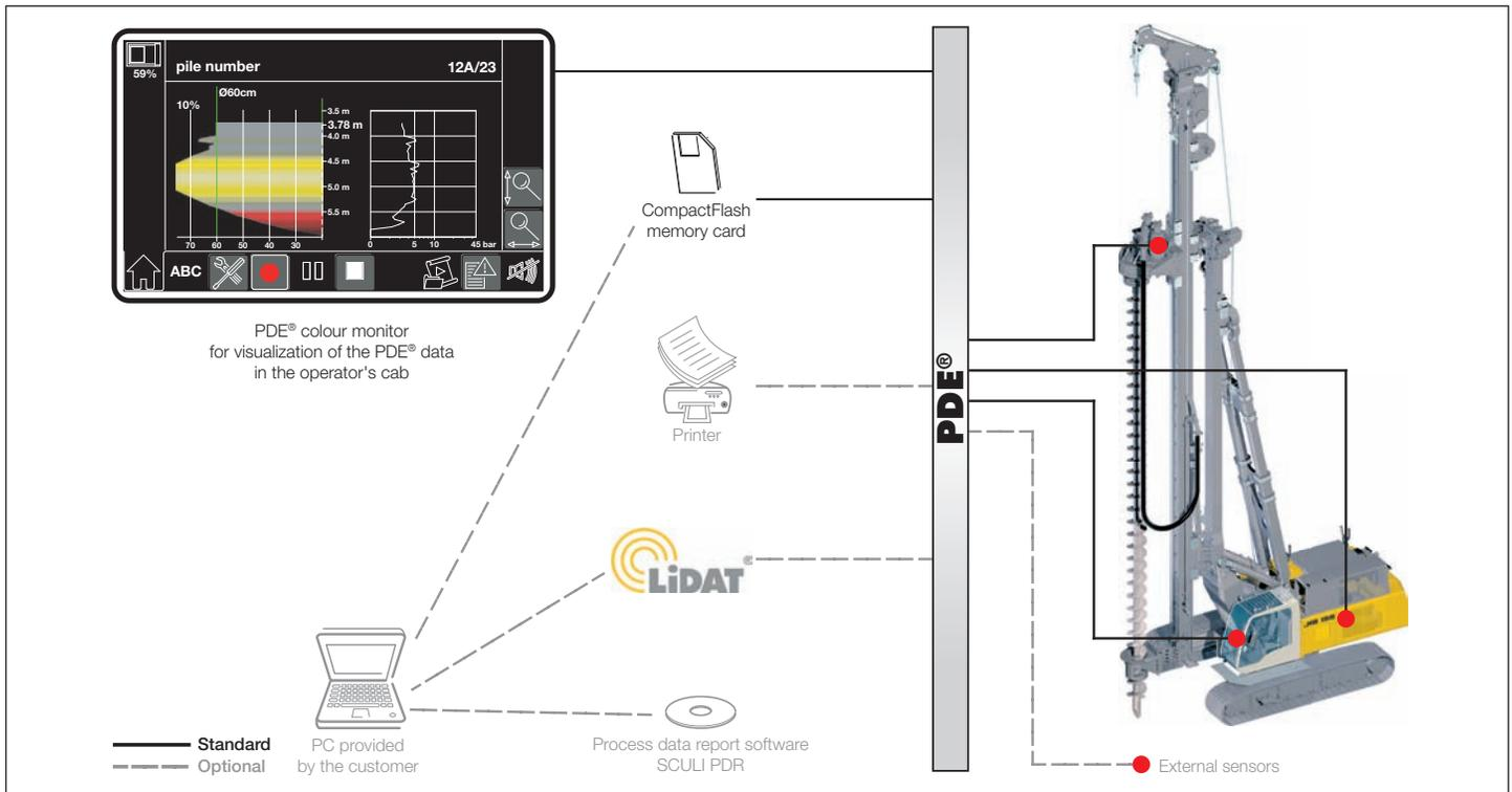
Depending on the application the recorded and processed data are displayed on the PDE® touchscreen in the operator's cab, e.g. in the form of an online cast-in-place pile.
