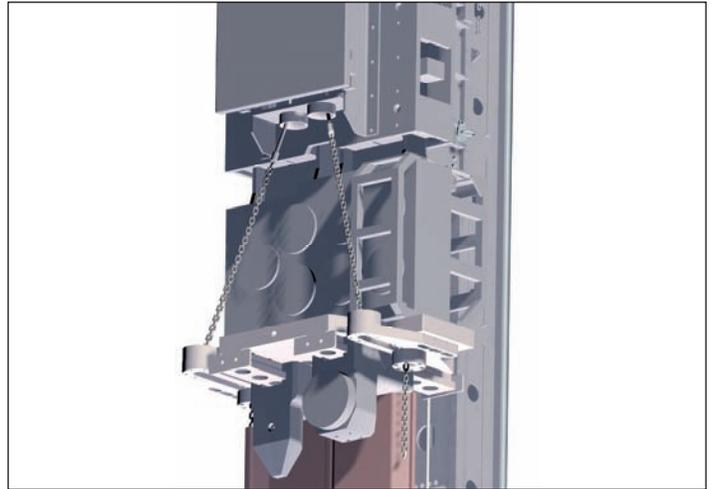
Double clamp and hydraulic sheet pile feeder
