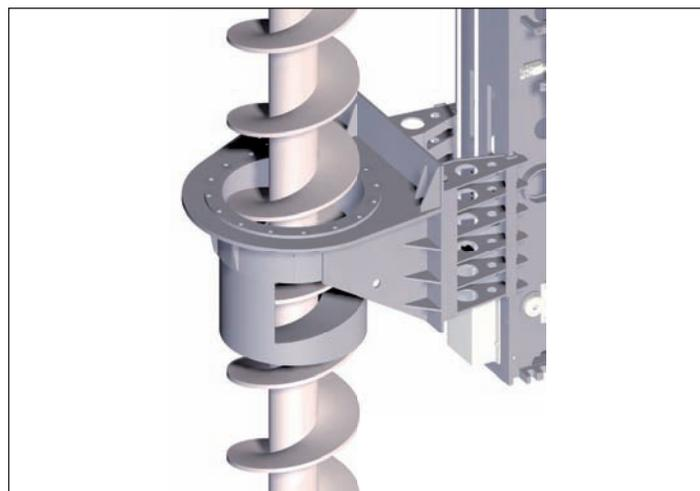
Auger with hydraulic auger cleaner
