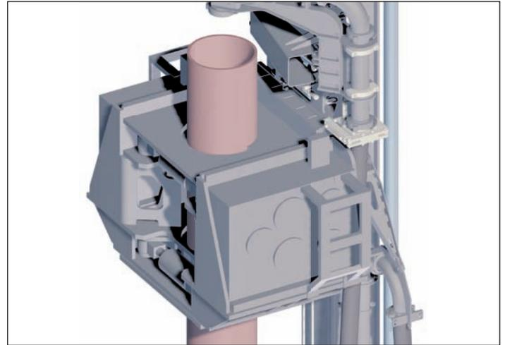
Ring vibrator with concreting system
