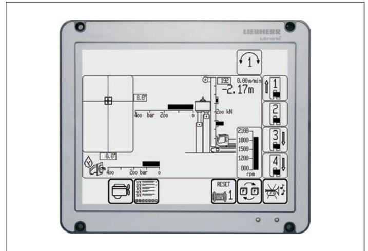
Display for sheet pile press
