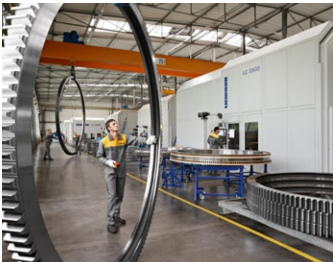
Large diameter bearing in production
