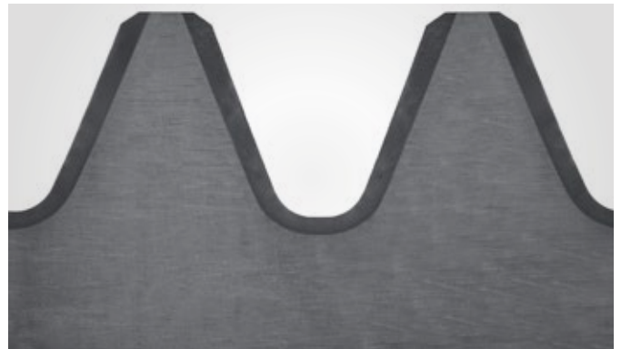
Hardening microsection of tooth spacing hardening
