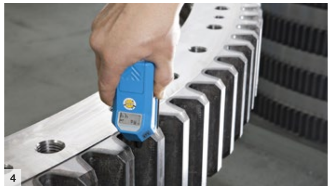
Surface inspection (surface roughness)
