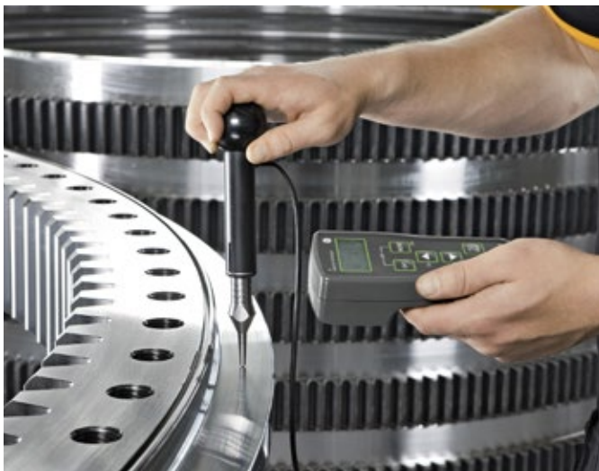
Quality check of large diameter bearings
