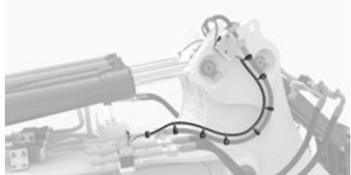
Cylinder dampening through IMUs provides smoother attachment movements without affecting attachment speed.
