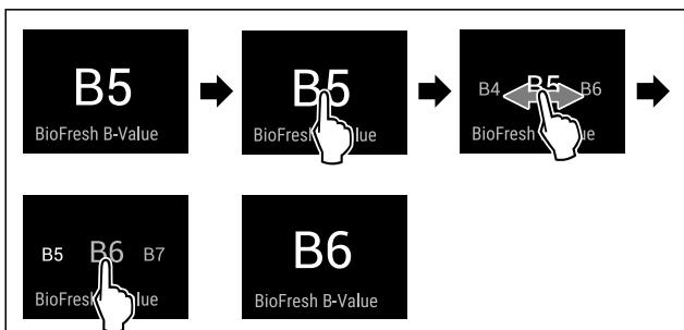
Fig. 27 Example illustration: Switch from B5 to B6.
