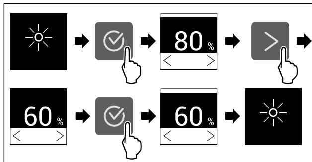
Fig. 49 Example illustration: Switch from 80 % to 60 %.
