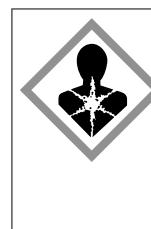
This symbol may be found on the compressor. It pertains to the oil in the compressor and indicates the following danger: Can be fatal if swallowed or with penetration of the respiratory tract. This information is only significant for recycling. No risk exists with normal use. Do not remove this symbol.
