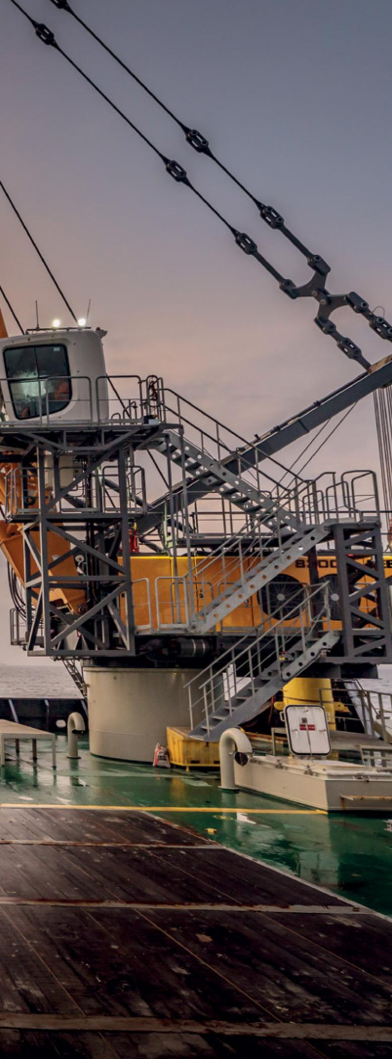
With an operating weight of 350 tonnes, the HS 8300.2 from Liebherr is one of the largest duty cycle crawler cranes available. It can be equipped with various high-volume dragline buckets and grabs.
