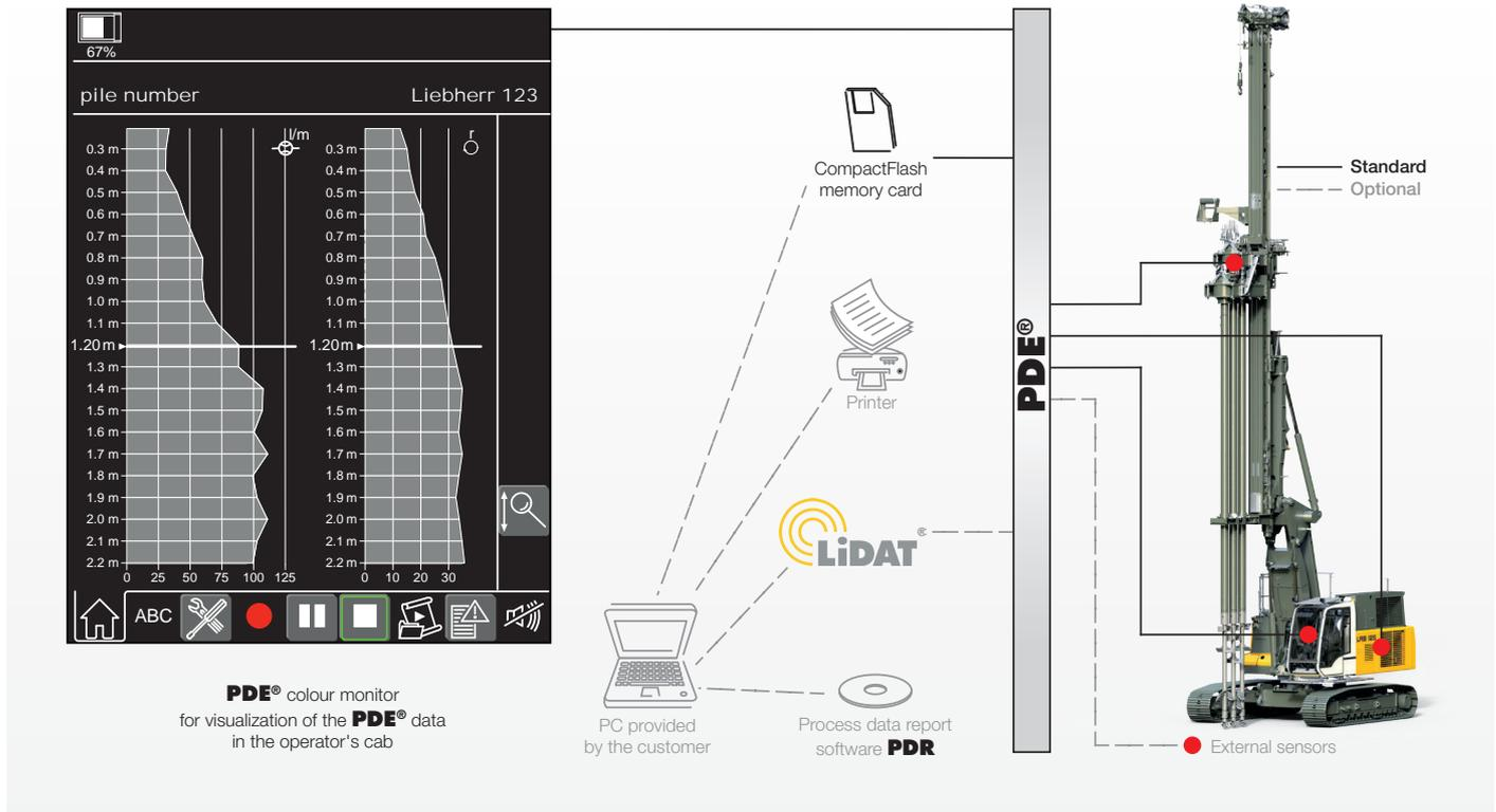
Depending on the application the recorded and processed data are displayed on the PDE® touchscreen in the operator's cab, e.g. in the form of an online cast-in-place pile.
