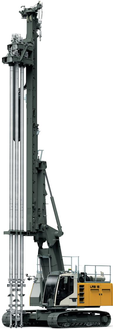
Max. drilling depth 14.9 m
