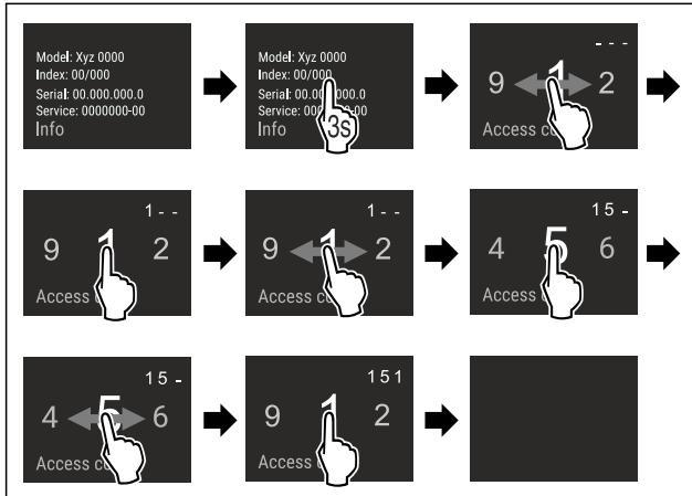
Fig. 5 Example illustration, access with numerical code **151**
