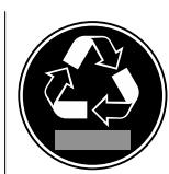
This or a similar symbol may be on the rear of the appliance. It indicates that there are vacuum insulation panels (VIP) or perlite panels in the door and/or housing. This information is only significant for recycling. Do not remove this symbol.
