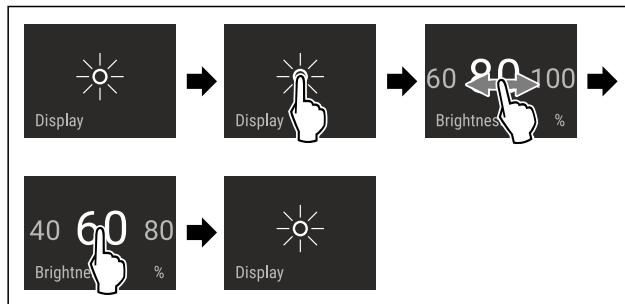
Fig. 45 Example illustration: Switching from 80 % to 60 %.
