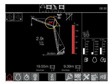
The crane operator receives a visual warning before reaching the tipping angle of the luffing jib's rigid tilting-back supports.
