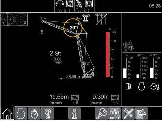
The crane operator sees the jib's negative angle on the monitor in real time.
