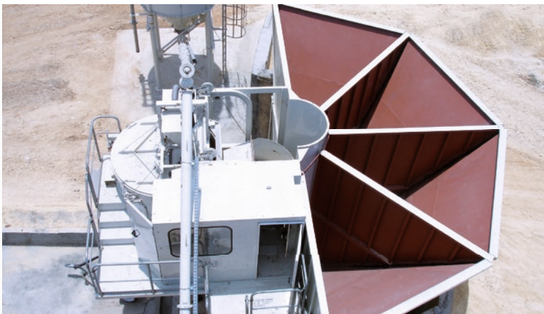
Design as star-pattern aggregate bays 4 compartments with total of 40 m 3 storage volume.
