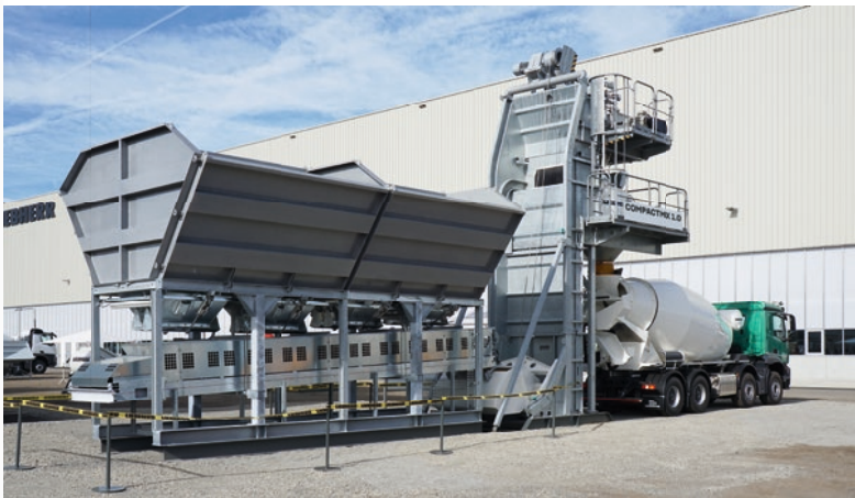
Design as mobile in-line silo (bin) 2 to 8 compartments possible with storage volume of 50 to 150 m 3 .
