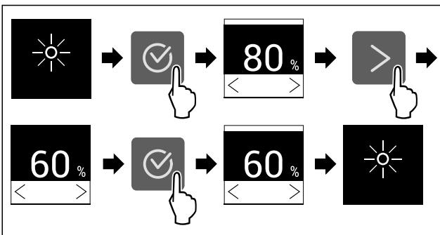
Fig. 46 Example illustration: Switch from 80 % to 60 %.
