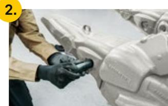
2. Remove the securing pin from the mounting.
