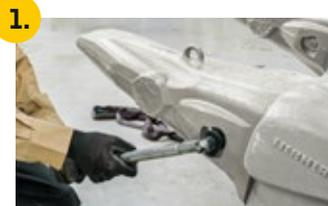
1. Unlock the securing pin with the locking spanner.
