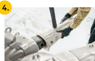
4. Slide the new tooth onto the tooth adapter.
