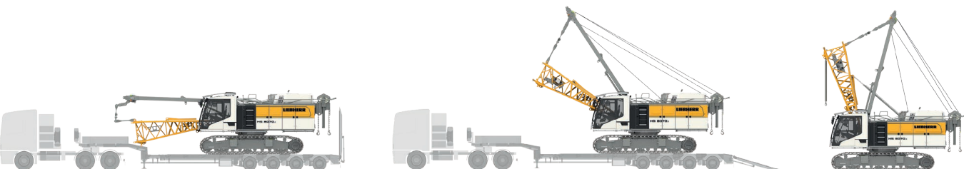
Unloading of basic machine (standard)
