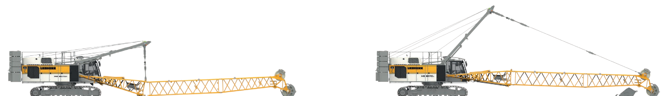
Assembly of boom and reeving of hoist ropes
