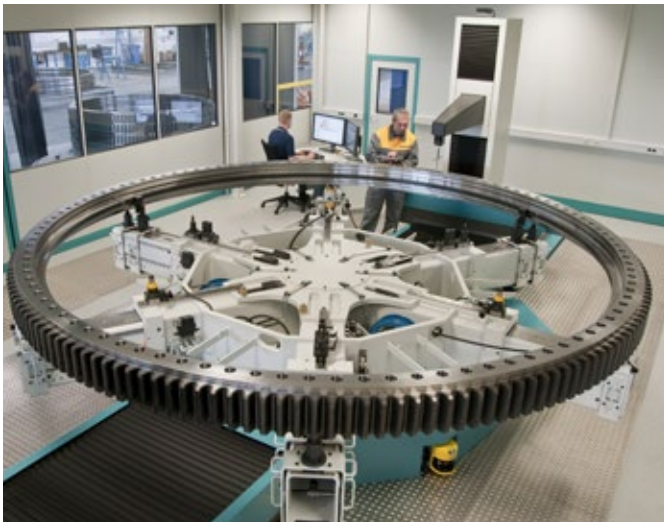
CMM machine for large diameter bearings
