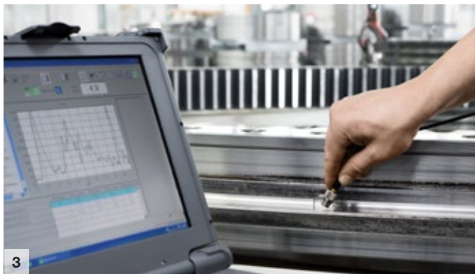
Measurement of hardness depth
