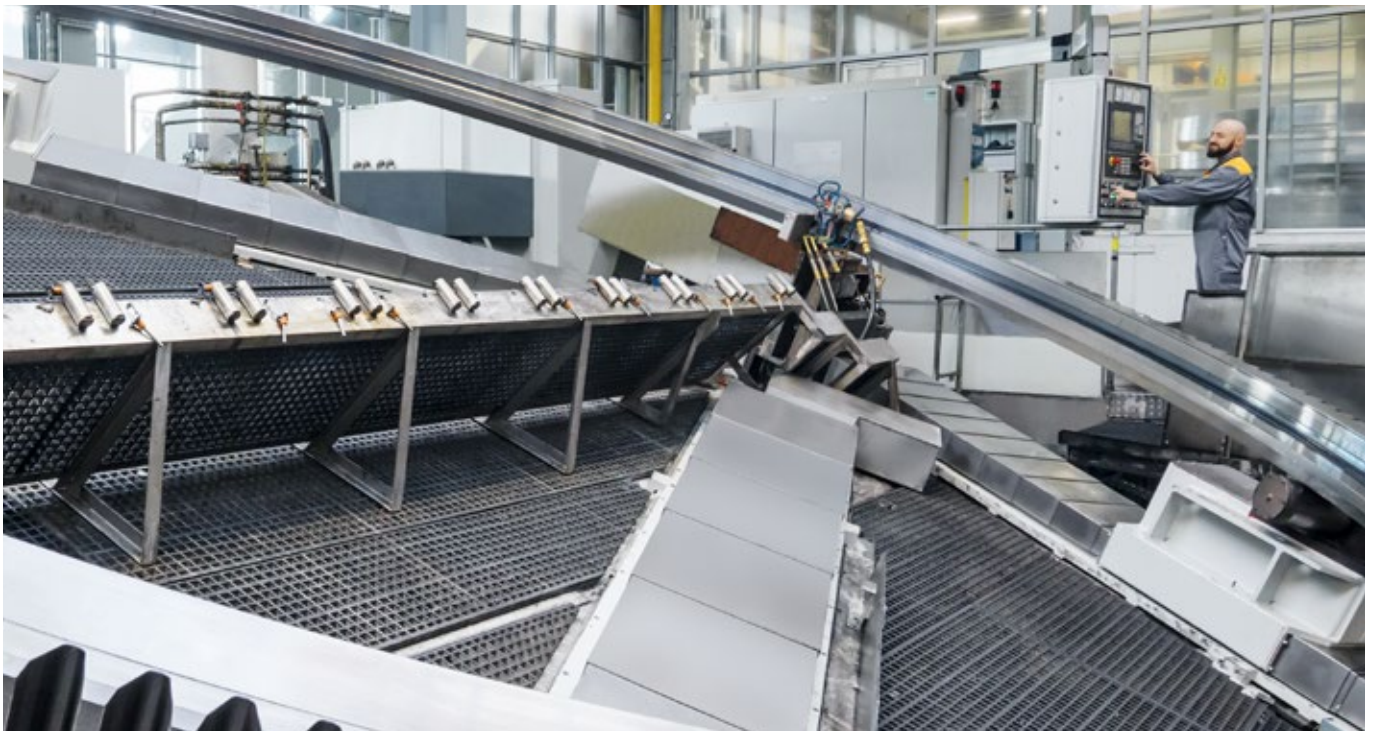
Induction hardening at Liebherr
