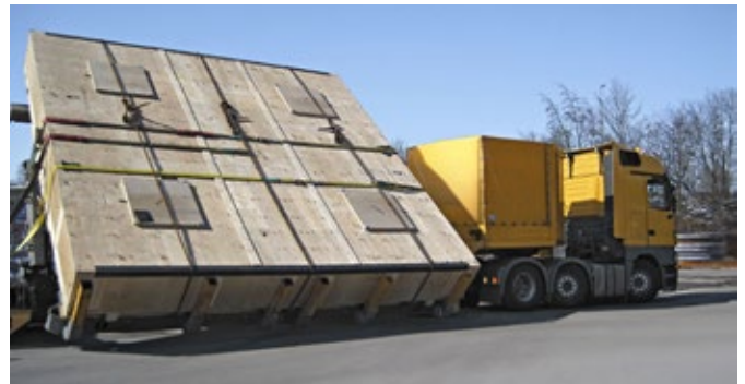
Low-loader with diagonal mounting
