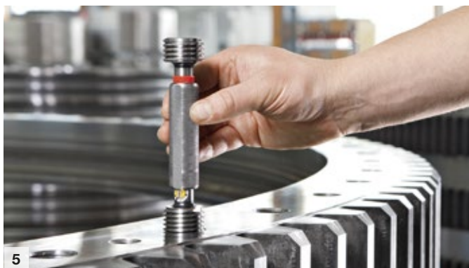
Dimension checks and visual inspection
