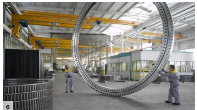
6 Completed large diameter bearing
