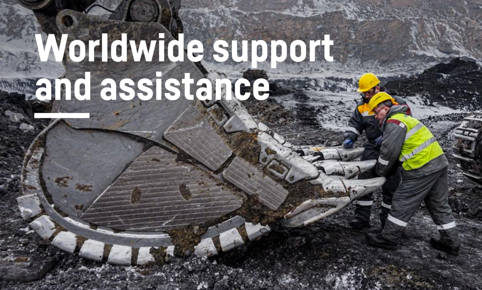
Routine assessments are conducted on all Liebherr buckets and Ground Engaging Tools (GETs) to detect signs of wear and understand maintenance requirements. The data collected during these inspections is meticulously recorded. Liebherr then uses the data to create detailed reports for customers that offer valuable operational insights and actionable recommendations for preventative maintenance measures.
