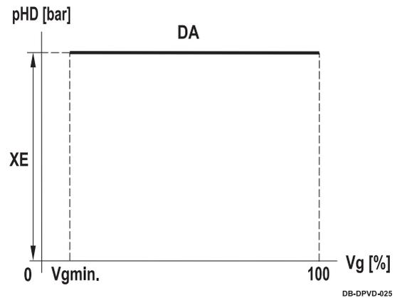
The DA pressure cut-off ensures that the maximum high pressure of the axial piston unit is limited within the regulation range. When a set high pressure value pHD is reached, the axial piston unit swivels in direction  $V_{g \min}$  and the hydraulic system is protected against damage and overloading.
