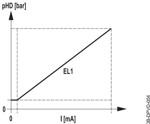
The EL function is designed with a positive characteristic as standard.
