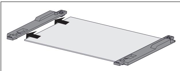
Fig. 109 Glass shelf with retaining part
