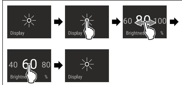
Fig. 44 Example illustration: Switching from 80 % to 60 %.
