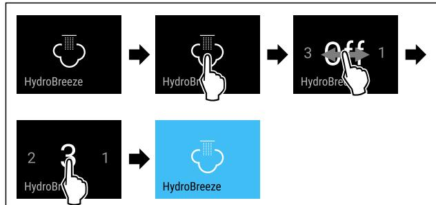
Fig. 37 Example illustration: HydroBreeze, activate with value 3.
