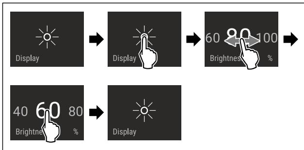
Fig. 56 Example illustration: Switching from 80 % to 60 %.
