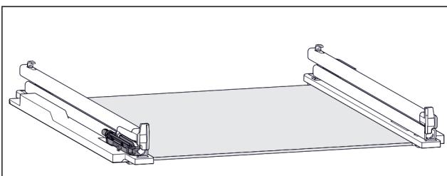
Fig. 111 Damping mechanism
