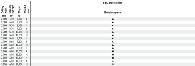
Level I: For non-abrasive materials, such as limestone without flint inclusion, shot material or easily breakable rock, i.e., deteriorated rock, soft limestone, shale, etc.
