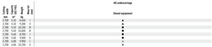
Level I: For non-abrasive materials, such as limestone without flint inclusion, shot material or easily breakable rock, i.e., deteriorated rock, soft limestone, shale, etc.
