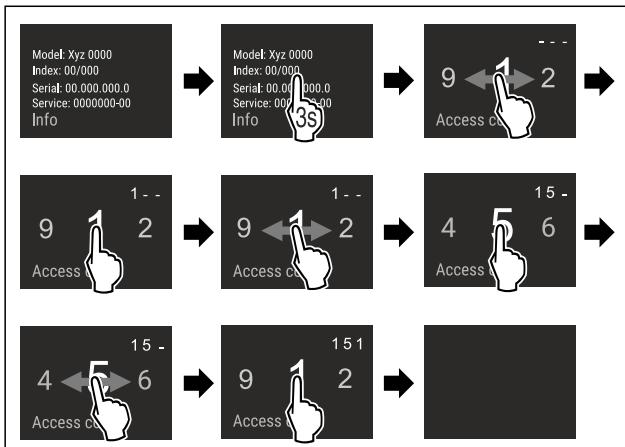
Fig. 4 Example illustration, access with numerical code **151**
