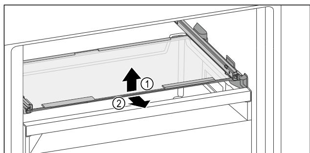
Fig. 107 Example illustration of the glass shelf\*
