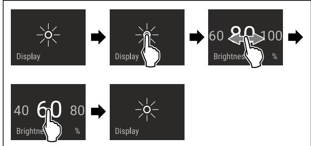
Fig. 48 Example illustration: Switching from 80 % to 60 %.
