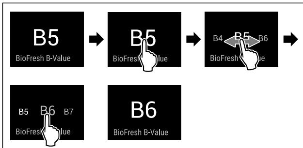
Fig. 24 Example illustration: Switching from B5 to B6.
