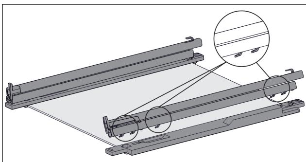
Fig. 124 Glass shelf with rails and retaining parts
