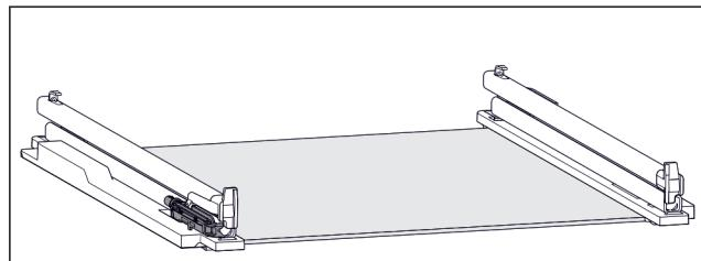
Fig. 127 Damping mechanism
