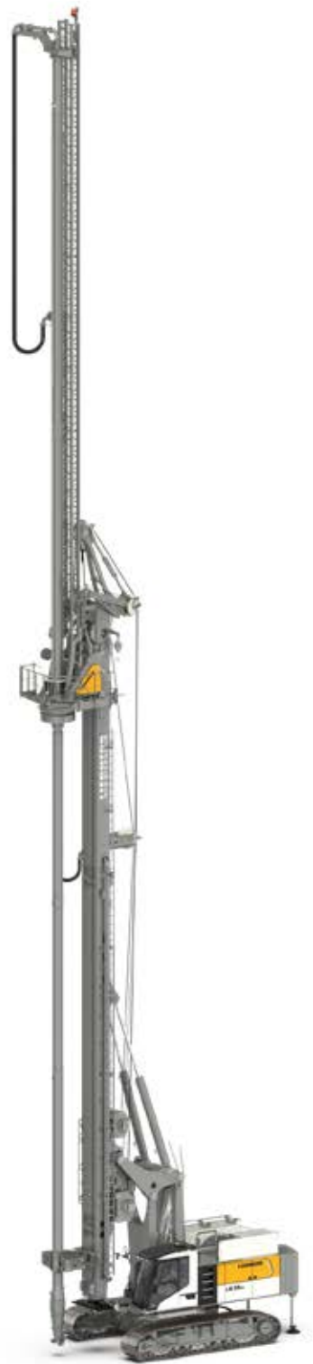
Full displacement drilling with lattice boom extension
