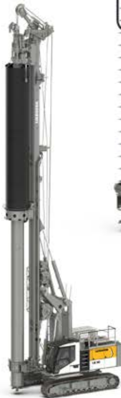
Continuous flight auger drilling with Kelly extension
