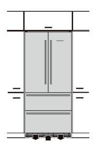
CBS 20 appliances don't need any ventilation openings in the cabinet. The required airfl ow is directed through the toe kick area.
