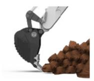
**Anti-stalling function**Prevents the bucket from being stalled during the digging phase.
