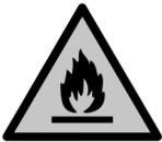
This symbol is located on the compressor and indicates the danger of flammable materials. Do not remove the sticker.
