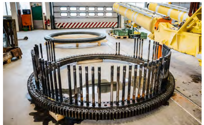
Slewing ring inspection with subsequent replacement
