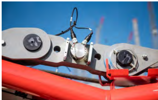
The load cell has a dual-channel design (2 plugs).
