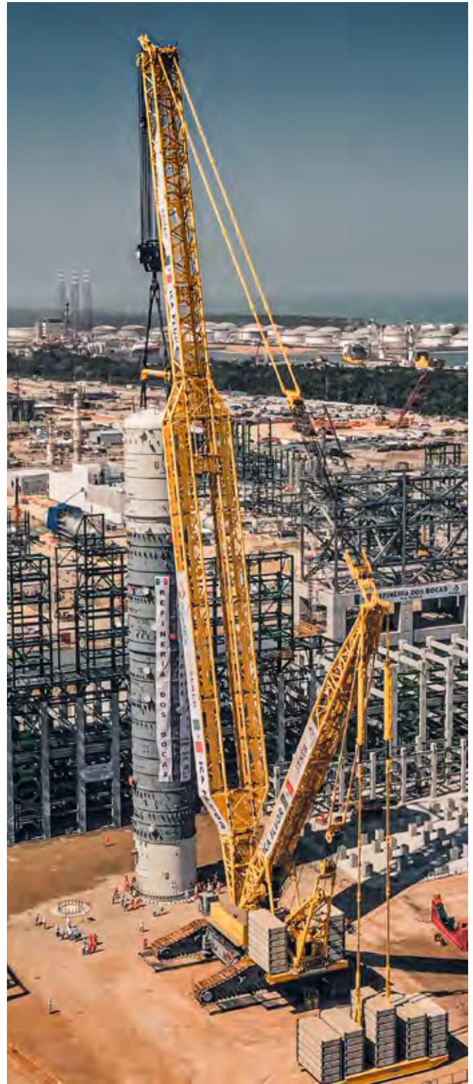
The PowerBoom parallel boom increases the rigidity of the boom enormously, enabling the LR 13000 to achieve particularly high lifting capacities.
