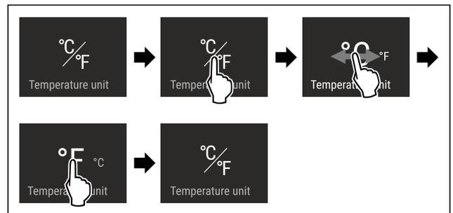
Fig. 18 Example illustration: Switch from degrees Celsius to degrees Fahrenheit.
