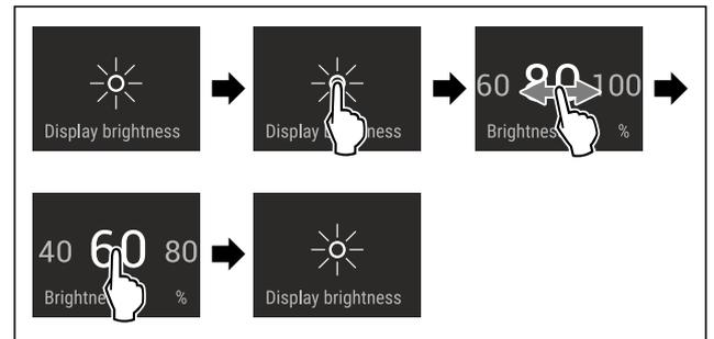
Fig. 32 Example illustration: Switch from 80 % to 60 %.
