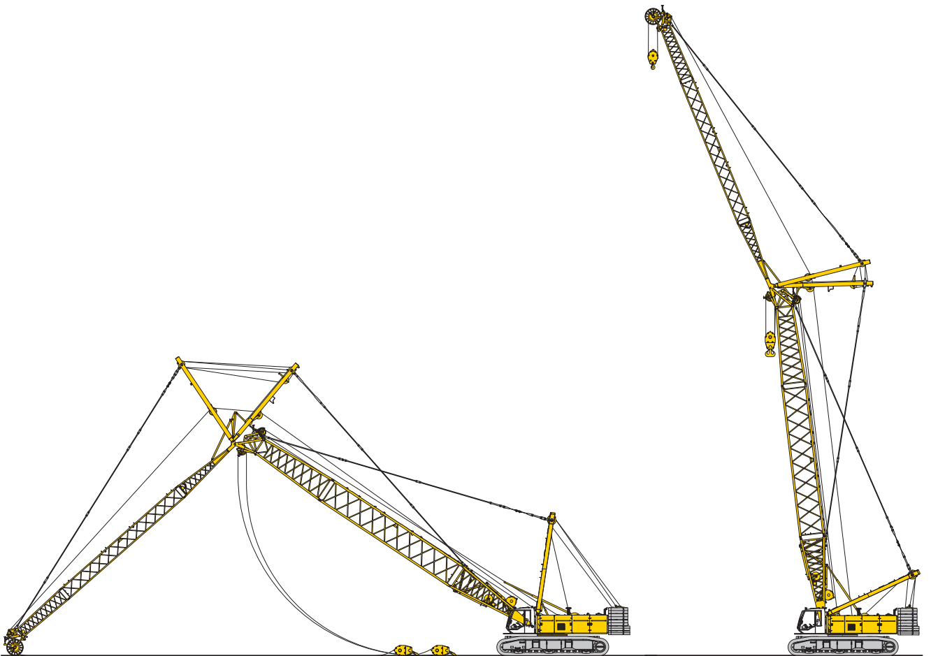
Erecting of main boom and luffing jib
