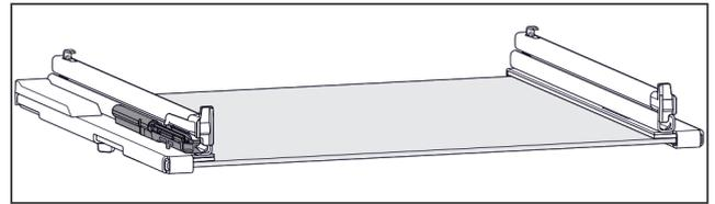
*Fig. 42 Damping mechanism*
