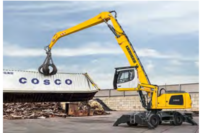
Container dismantling with the LH 40 M Industry Litronic
