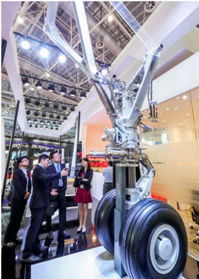
Impressive trade show exhibit: the nose landing gear of the A350 XWB
