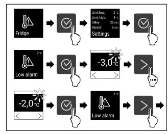
Fig. 138 Example of setting the lower temperature limit based on a set appliance temperature of 5 °C.
