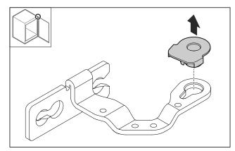
► Press out the bearing socket.
