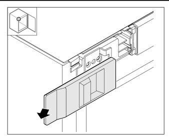
Fig. 12 ► Remove the cover.
