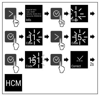
Fig. 5 Access with numerical code 151
