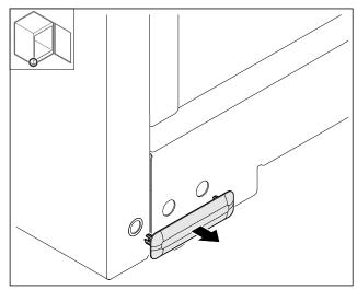
Fig. 14 ► Remove the cover.
