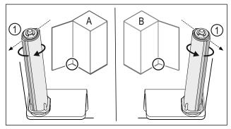
Fig. 45 Left stop (A) / right stop (B)
