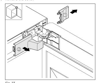
Fig. 13 ▶ Remove the cover Fig. 13 (1) and then Fig. 13 (2).
