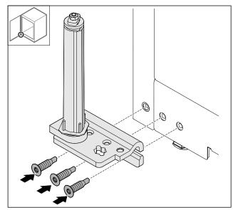
▶ Attach the hinge bracket on the opposite side.
