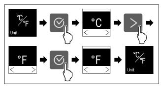
Fig. 94 Example illustration: Switch from degrees Celsius to degrees Fahrenheit.
