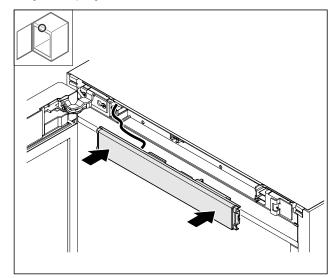
Fig. 50 ▶ Put on the front panel.
