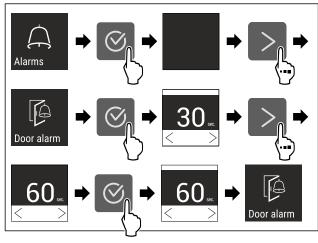
Fig. 148 Example illustration: Switch door alarm from 30 seconds to 60 seconds.
