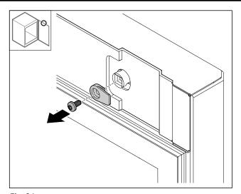
Fig. 26 ► Detach the locking hook.
