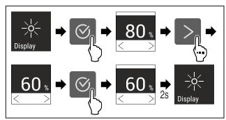
Fig. 96 Example illustration: Switch from 80 % to 60 %.
