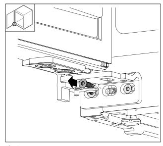
Fig. 56▶ Remove the middle screw on the lower hinge.
