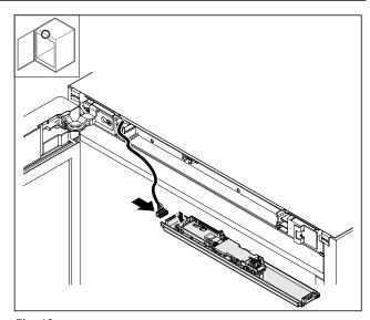
Fig. 49 ▶ Plug in the plug.
