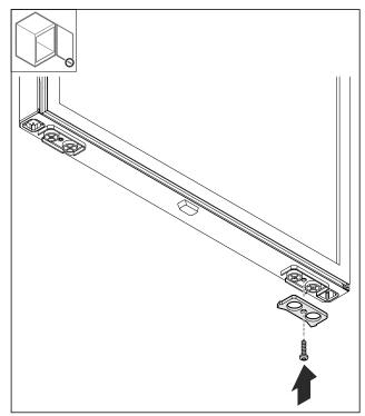
Fig. 23 ► Attach the stop plate on the opposite side.
