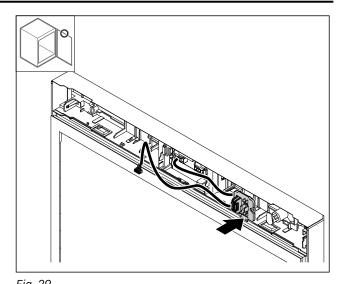
Fig. 29 ► Engage the plug holder on the opposite side.
