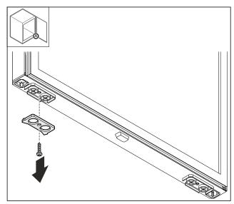
Fig. 22 ▶ Detach the stop plate.
