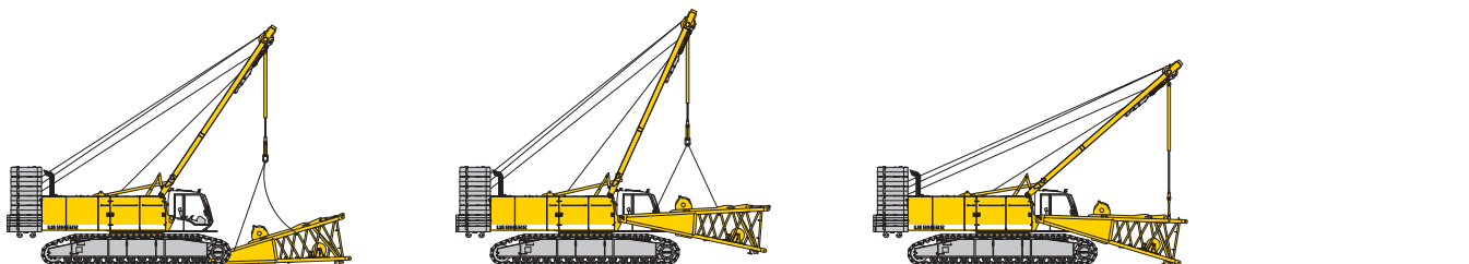
Unloading and assembly of boom foot
