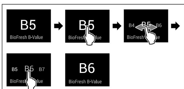
Fig. 25 Example illustration: Switch from B5 to B6.
