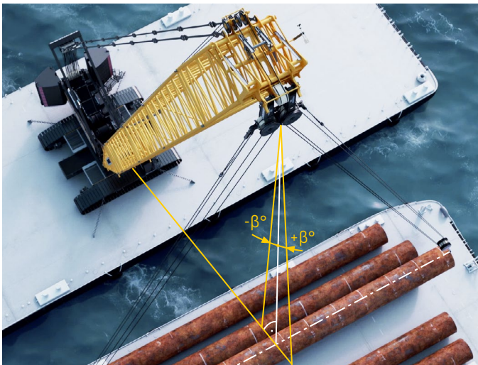
Optional Off-lead Compensation: At the touch of a button, the diagonal pull in the boom direction and thus the load swing in the boom direction can be avoided.
