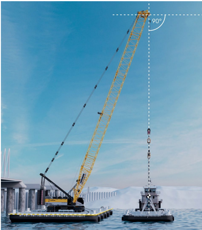
At the touch of a button, the boom head positions itself above the load's centre of gravity. This prevents diagonal pull and the load can be lifted without swinging.
