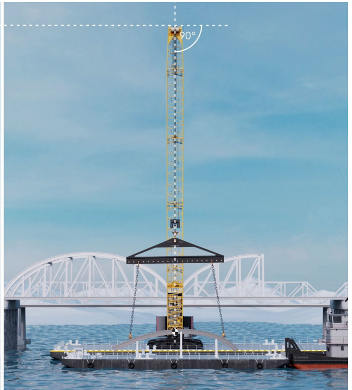
At the touch of a button, the boom head positions itself above the load's centre of gravity. This prevents diagonal pull and the load can be lifted without swinging.
