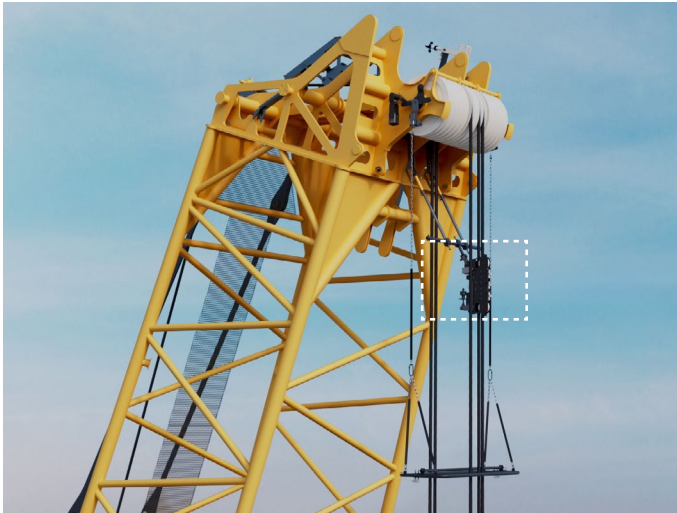
Sensors determine the rope lead-off angle
