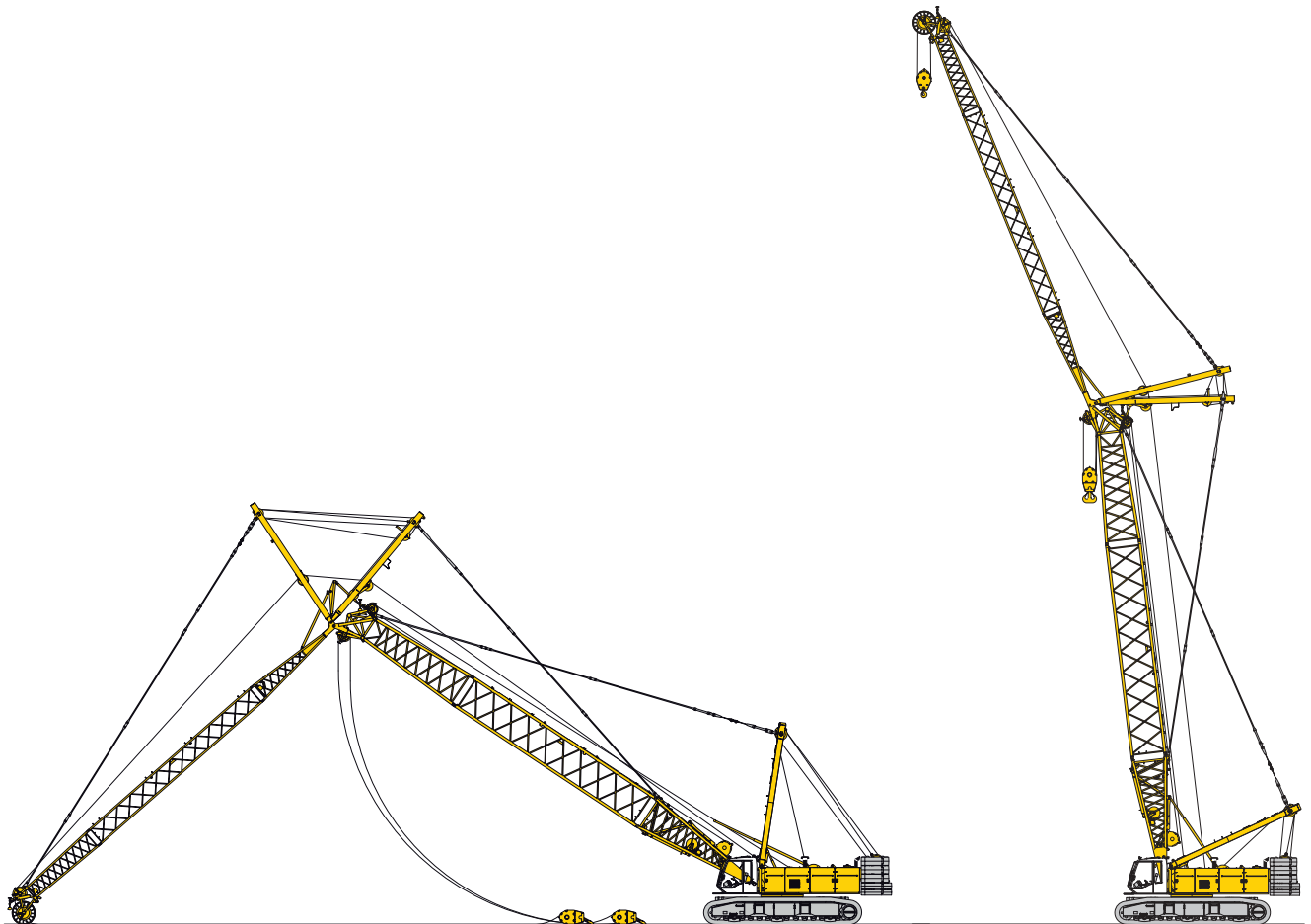
Erecting of main boom and luffing jib
