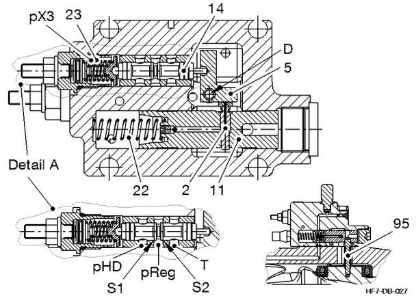
Override: The external control pressure  $pX3$  is directed to the LR control axis via port X3 and acts against a measuring piston in addition to the spring force of the LR control. To maintain the force balance, the axial piston unit swivels towards  $V_{g \max}$  to a higher performance level.
