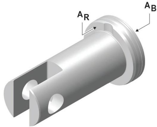
If the EL function is designed with a negative characteristic, the axial piston unit swivels towards a larger displacement volume  $V_g$  as the control current  $I$  decreases. The high pressure  $p_{HD}$  is applied to the adjusting piston ring area  $A_R$ , and the regulated high pressure  $p_{Reg}$  is applied to the adjusting piston bottom area  $A_B$ .
