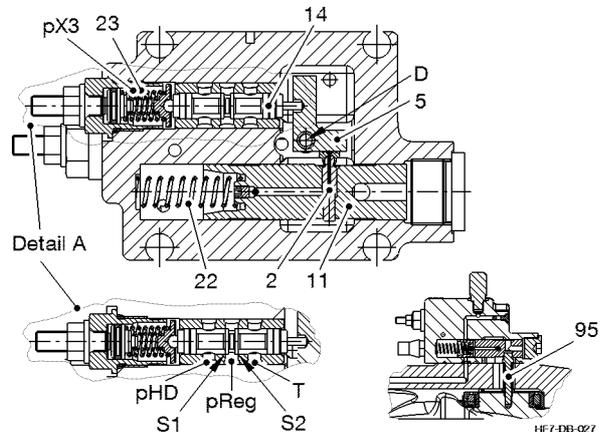
The LR function adjusts the flow rate  $V_g$  (volume flow) of the axial piston unit, depending on the pump high pressure pHD (the capacity reduction), to the performance characteristic of the drive motor while limiting the flow at a constant speed  $n$ .
