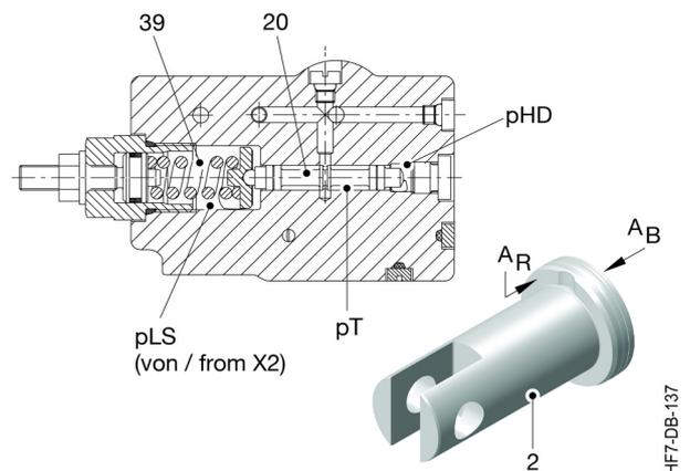
The dynamic characteristics of the control system of variable hydraulic pumps can be further improved by load sensing (LS) systems, such as an EL/LS control. The LS function is designed as a so-called load pressure reporting system that adjusts the pressure and volume flow to the current requirements of one or more consumers.
