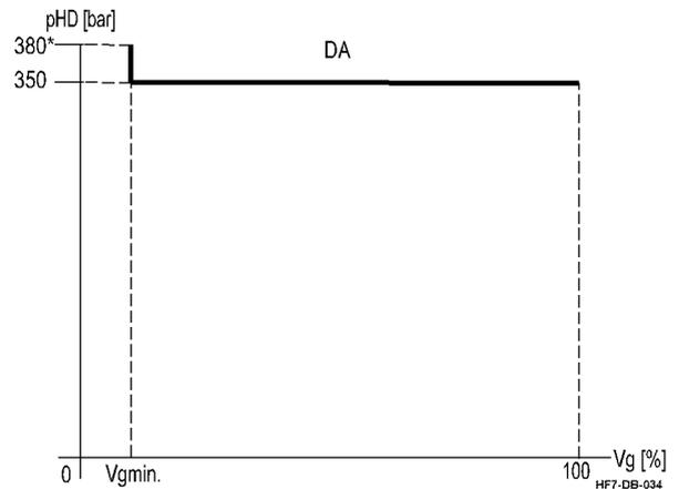
DA pressure control minimizes or limits (cut-off) the volume flow of the axial piston unit, when a fixed high pressure value pHD is reached. Swivelling in the direction of  $V_{g \min}$  protects the hydraulic system from damage and overload.
