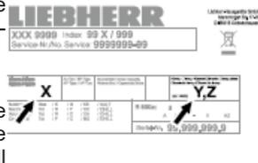
The climate class [Y] and temperature class [Z] define the maximum outline conditions in which the appliances will operate perfectly
