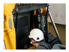
Simple cleaning of the radiator Liebherr crawler dozers are fitted with a swivelling fan as standard and with a quick-release fastener as an option. This allows cleaning from the outside in double-quick time. An optional reversible fan is recommended for self-cleaning, particularly in dustintensive applications.
