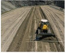
Assistance systems as standard "Free Grade" and "Definition Grade" assistance systems make life easier on road construction, maintenance or mining operations. And they come fitted as standard – without complex 3D machine control.
