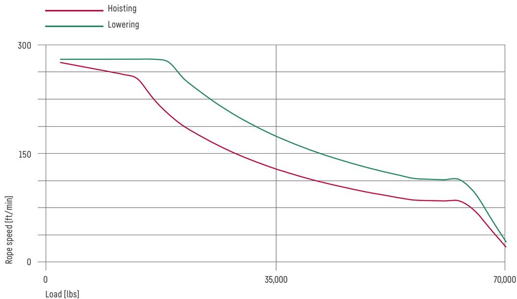
Diagram shows the course of a winch in dual-winch operation
