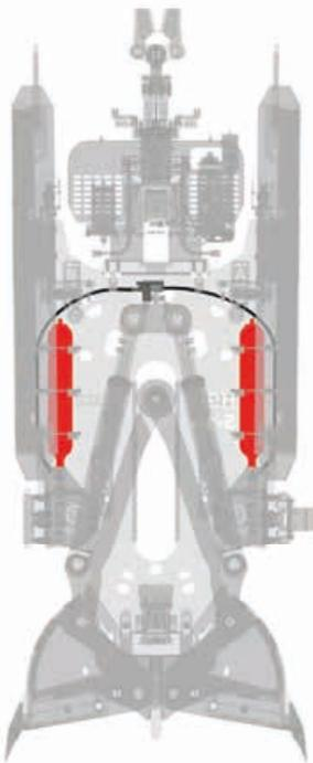
These additionally installed accumulators temporarily store the high oil flow that occurs when the jaws are opened. As a result, high opening and closing speeds can be achieved despite generously dimensioned cylinders.
