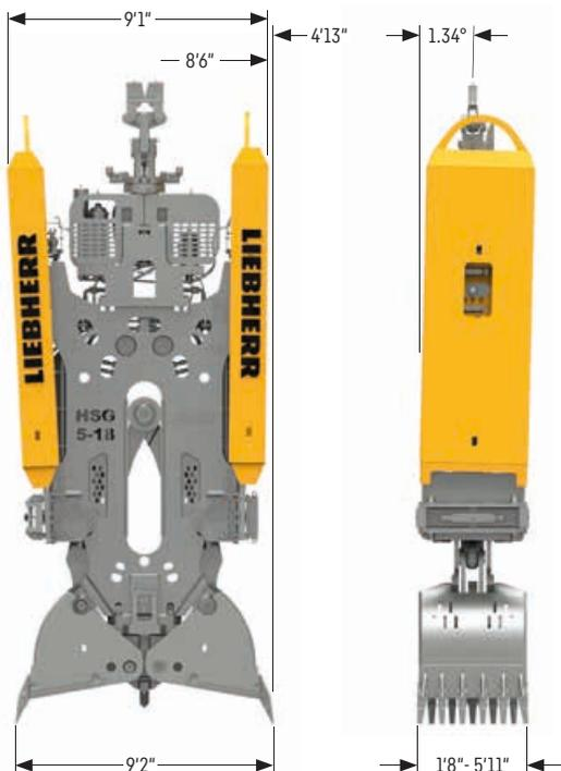
During excavation work the grab direction can be corrected using the guide bars and so higher verticality of the slurry wall is achieved. The system is driven hydraulically and can be controlled from the cabin.
