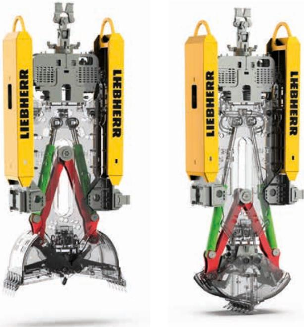
Opening and closing of the grab is actuated by two direct-acting cylinders. These are installed with the piston rods at the top, which means they are protected inside the grab body. The robust cylinder barrels are positioned downwards.
