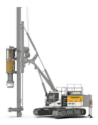
By supporting the leader on the ground and extending the rear support cylinders, the carrier machine is elevated. The undercarriage can thus be swivelled on the spot, which makes it easier to move the piling rig in restricted spaces.
