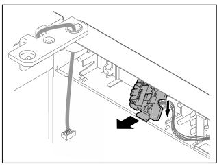
Fig. 24 The installation position of the plug holder can be rotated by 180°.
