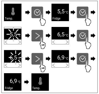
Fig. 71 Changing temperature from 5.5 °C to 6.9 °C
