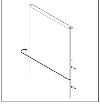
Fig. 34 Put the stopper on the opposite side.
