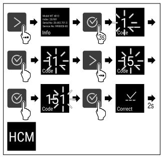
Fig. 6 Access with numerical code 151
