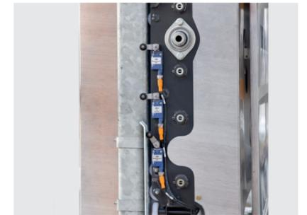
The central limit switch cuts out only in an emergency
