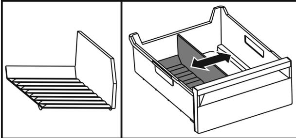
Fig. 69 Example illustration of the ice compartment divider
