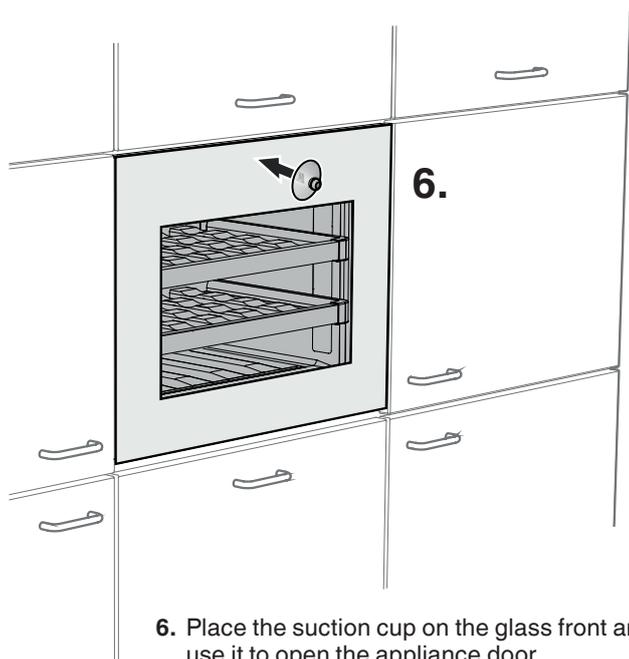
6. Place the suction cup on the glass front and use it to open the appliance door.
