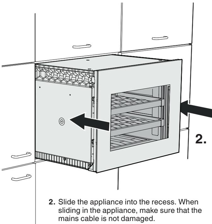
2. Slide the appliance into the recess. When sliding in the appliance, make sure that the mains cable is not damaged.
