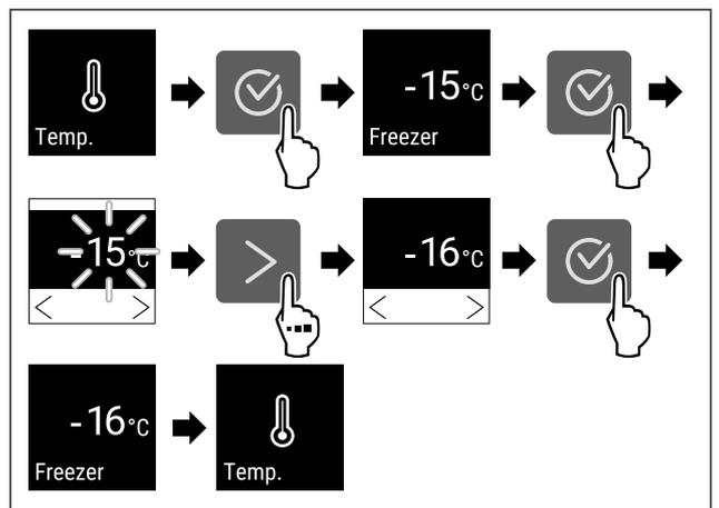
Fig. 59 Changing temperature from -15 °C to -16 °C
