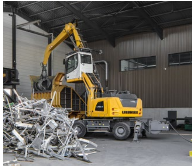
LH 26 M Industry E Litronic in scrap handling at MTB Recycling in Trept, France.
