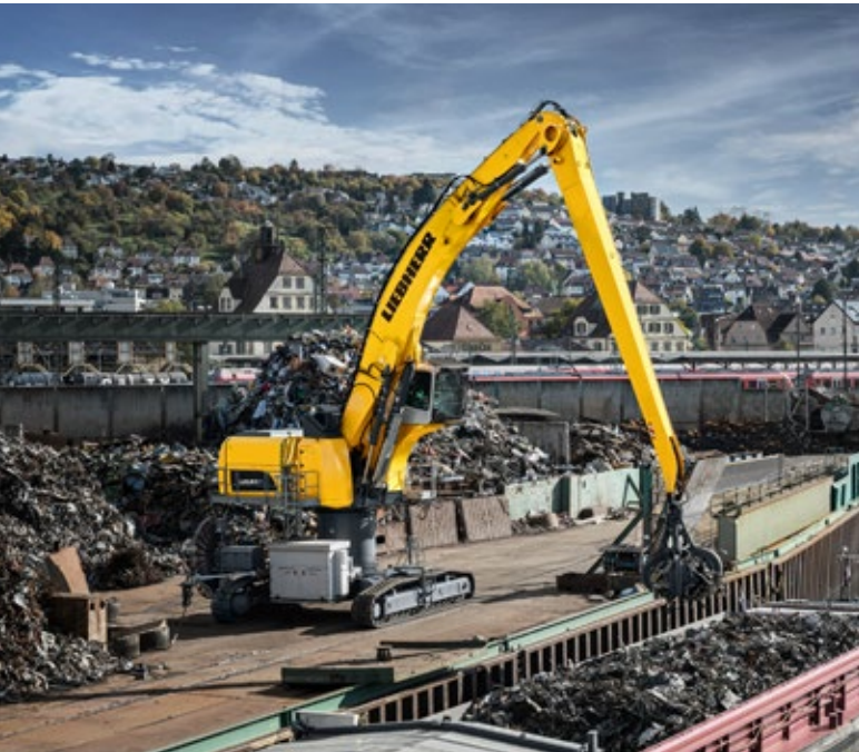
LH 150 C High Rise Industry E Litronic in scrap handling at Schrott- und Metallhandel M. Kaatsch GmbH in Plochingen, Germany
