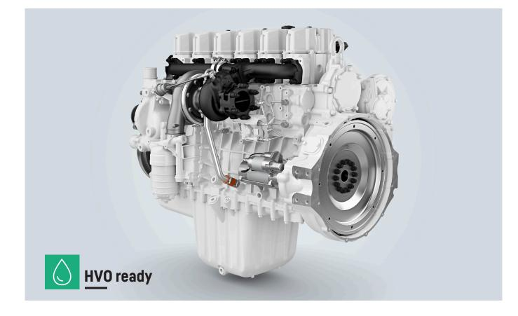
Liebherr's D966 is a very compact six-cylinder in-line engine. The robust design of the D966 is built to withstand the harshest conditions of the agriculture industry. This sixcylinder engine comes with an integrated centrifugal water pump and closed crankcase ventilation system, ultra fine fibre oil filter, fuel fine filter on engine as well as twin scroll turbocharger that considerably improve fuel consumption.
