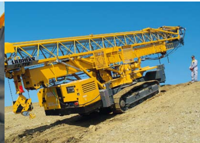
On the rise: Crawler cranes on the move with gradient inclinations of 30%.
