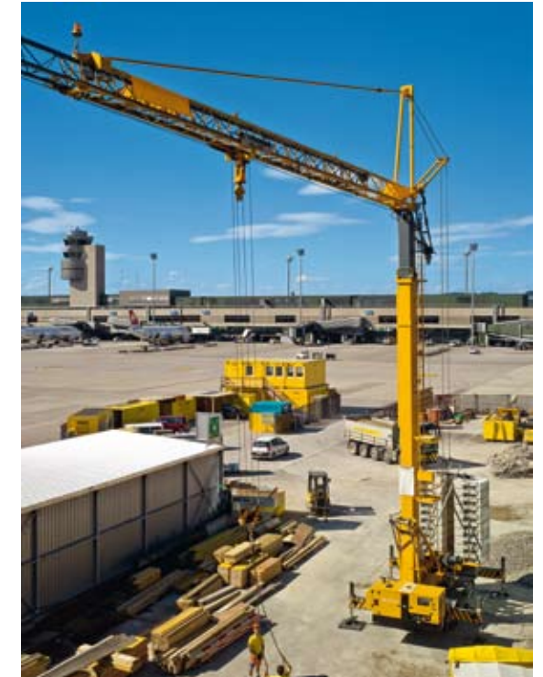
Flexible: The 32 TTR – maximum possible adaptability thanks to telescopic tower and jib.
