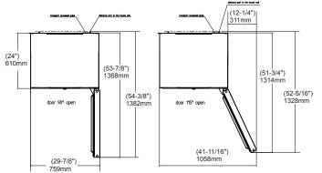
Allow door swing clearance at locations next to a wall. If the appliance is installed with the hinges next to a wall (4), the distance between the appliance and the wall must be at least  $\frac{1}{2}$ " (13 mm.)
